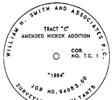
"TYPICAL" BOUNDARY MONUMENT TYPICAL 1/2" BRASS CAP ATTACHED TO A 2 1/4" DIAMETER BY 30" LONG IRON PIPE.
