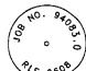
"TYPICAL" LOT CORNER TYPICAL 1/2" DIAMETER ALUMINUM CAP ATTACHED TO A 5/8" DIA REINFORCEMENT ROD.
