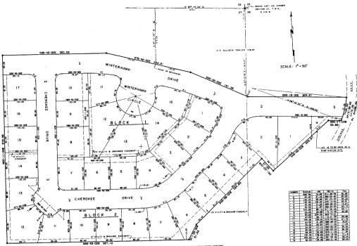
BEARINGS BASED ON UPCC TRIANGULATION SYSTEM 0 - DENOTES 5/8" x 18" REBAR WITH ALUMINUM CAP
